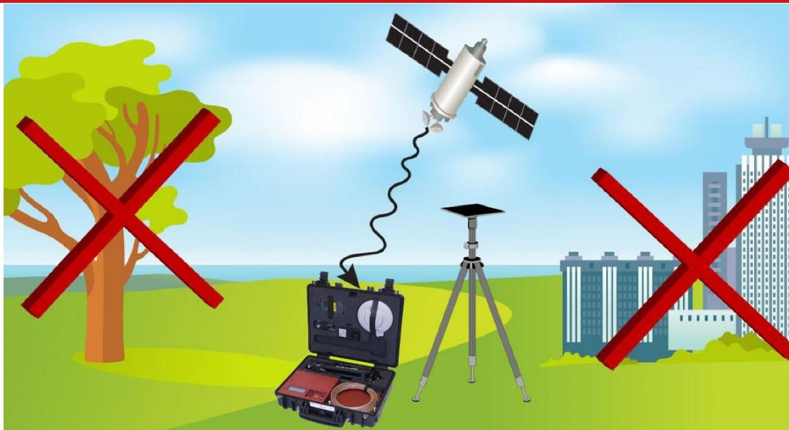
Choose a location for the GNSS antenna that is not close to buildings or trees, as these can both affect GNSS signals. The antenna needs to have a good view of the sky (not just above, but to the sides too).
