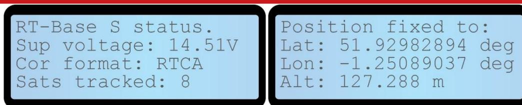
The LCD alternates between the two screens above at eight second intervals once a position has either been averaged over the specified time period, or a saved location has been loaded.
