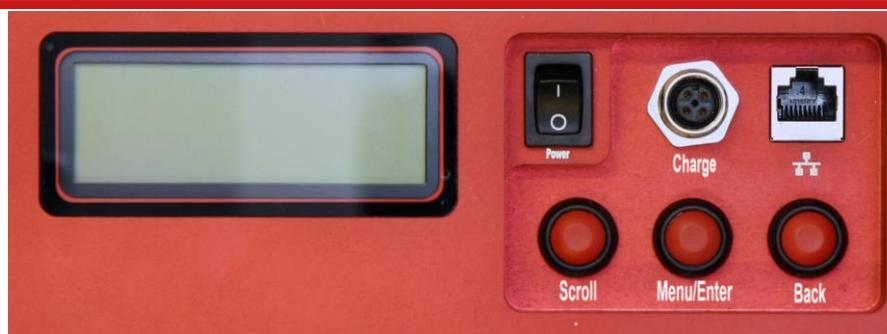
When power is first applied, the LCD shows the firmware version running in the RT-Base S along with the static IP address the unit is using to communicate (Figure 7). This information page is displayed for 10 seconds.
