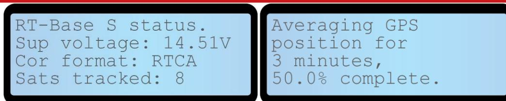
The LCD alternates between the two screens above at eight second intervals while it averages a position. This process can be interrupted at any time and a saved position can be loaded.
