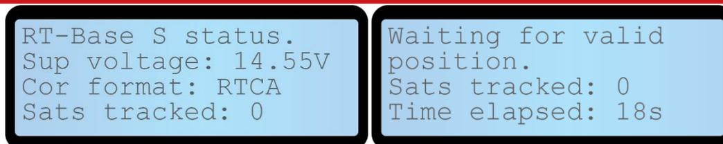
The LCD alternates between the two screens above at eight second intervals while it looks for a valid GNSS position.
